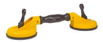
Makes working with unwieldy parts quicker and more effective  $\cdot$  suitable for all materials with smooth, flat, airtight surfaces such as glass, plastic, metal, coated wood and marble  $\cdot$  The longitudinal holes in the articulated joints (MM VER 602.22) allow transporting surfaces which are curved beyond standard  $\cdot$  suction discs: Ø 120 mm
